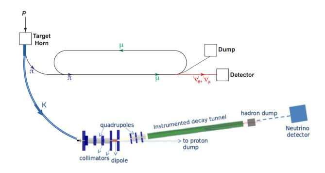
Conceptual layout that allows parallel running of both nuSTORM and ENUBET experiments
