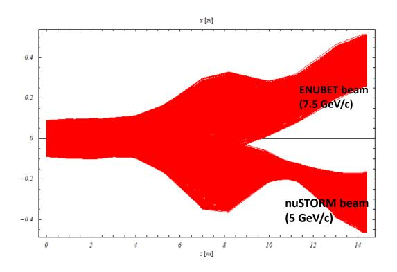
Tracking ~1000 particles along the common transport line with small momentum spread (1%). The chromatic effects are obvious for the two beams at the end of common transport line.
