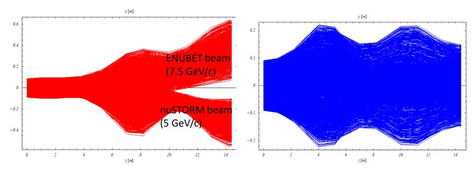
Tracking ~1000 particles along the common transport line with large momentum spread (10%). The initial alpha and beta are assumed to be the same. Good beam separation was achieved.
