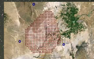
Telescope Array Surface Detector (covers ~700km 2 , 1.2km spacing of detectors)
