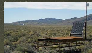
Each detector has 2 layers of 1.2cm thick plastic scintillator. Real-time calibration.
