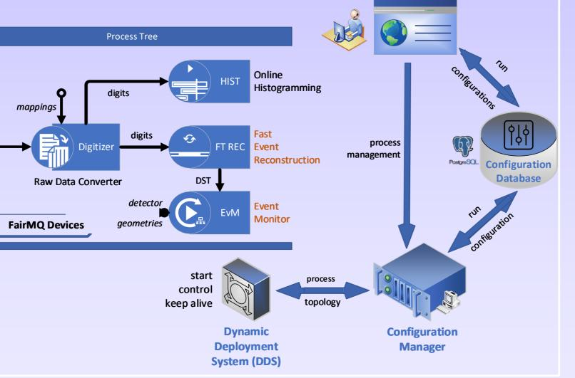
The DDS system has been chosen and is used by the Configuration Manager to start and manage processes.
