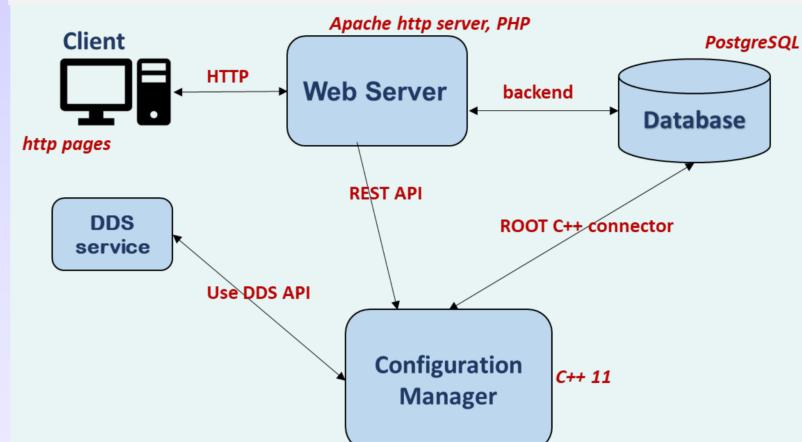
The **Configuration Manager** is responsible for starting, stopping and supervising tasks. It runs as a daemon process and performs obtained commands from the Web server using the **DDS** service that communicates with the DDS server via the C++ DDS API. Furthermore, the **Configuration Manager** reads data from the database and writes the necessary information concerning started, crashed or stopped tasks using the ROOT C++ connector.
