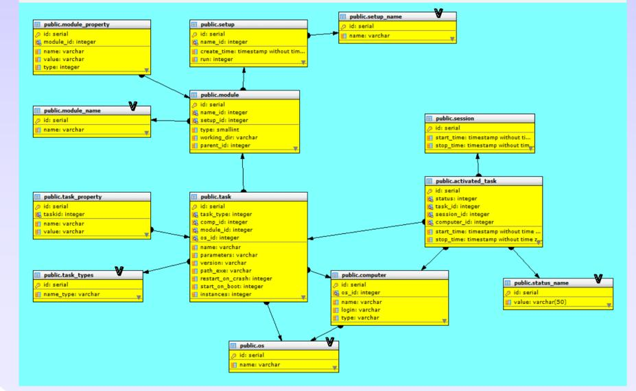
The *task* object of the *module* comprises all the attributes sufficient to start the task with the required parameters. The *task* also has a reference to the operating system object (os) to ensure that the task can be launched on a given computer. The reference to the *computer* object sets a host, on which the task will be started. The operating system installed in the computer is defined by a reference to the **os** object.
