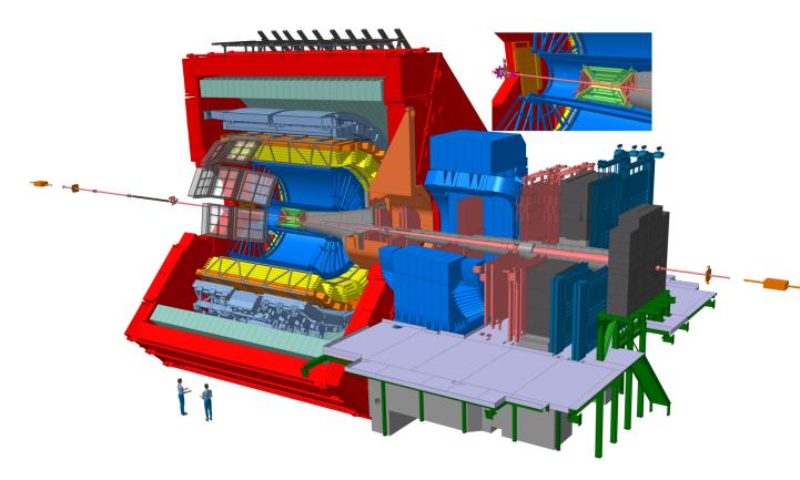
**Specificity:** low-momentum tracking and particle identification in a highmultiplicity environment
