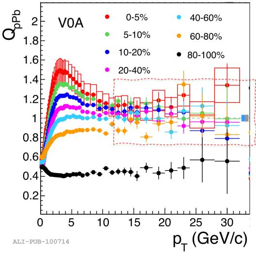
The Q<sub>pPb</sub>: the nuclear modification factor in multiplicity classes in p-Pb
