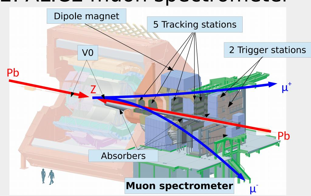
**Absorber system:** Stop  $\pi$ , K and low momentum  $\mu$ **Dipole magnet:** Integrated field strength of 3 Tm Muon tracking chambers: Reconstruct charged particle tracks
