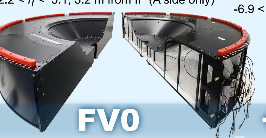
plastic scintillator connected with clear fibers to 48 fine-mesh PMTs (Hamamatsu R5924-70)
