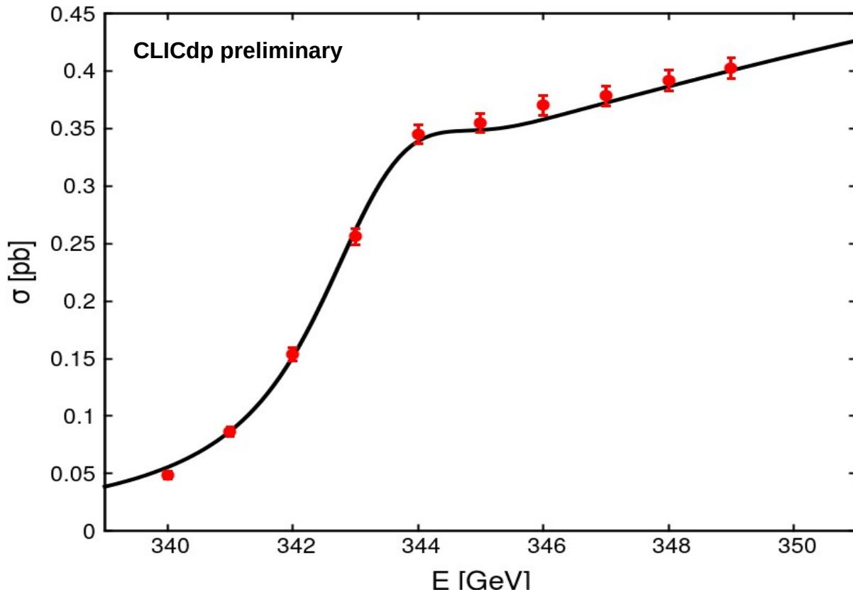
Generate statistical fluctuation assuming 70.2% event reconstruction efficiency and background level (remaining after cuts) corresponding to the 73 fb
