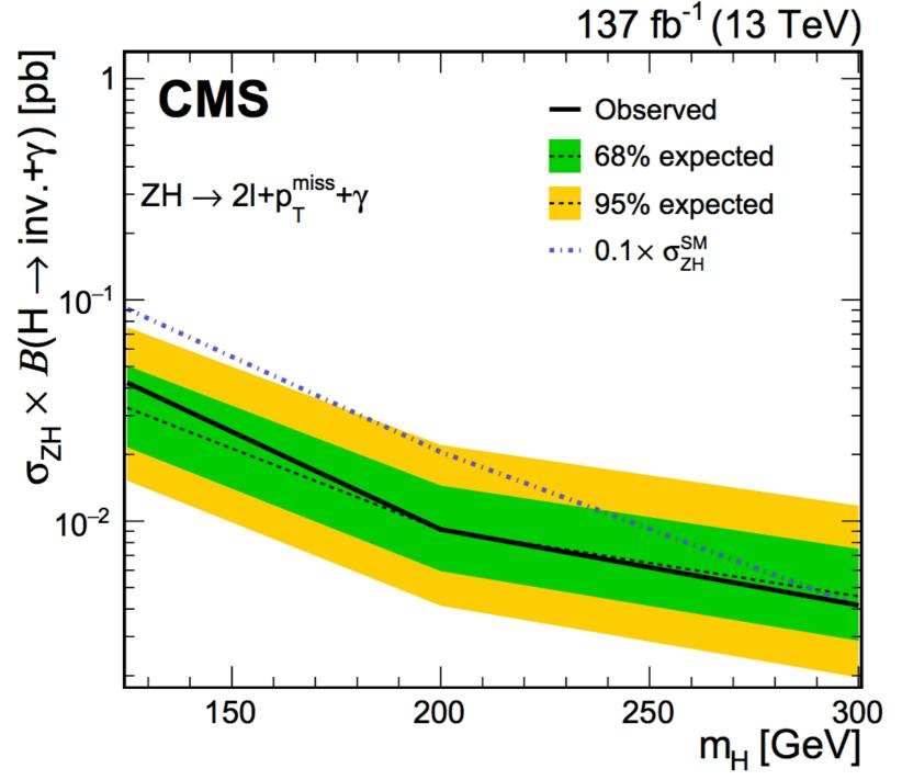
Statistical uncertainty dominates. Systematics due to PDF choice, jet energy scale, object reconstruction/ identification efficiency, integrated luminosity etc taken into account.
