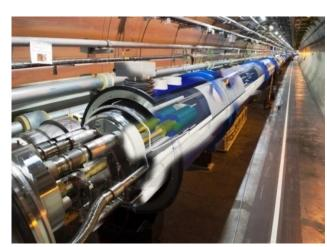
1232 Main Dipoles + 448 Main Quadrupoles cooled by 120 Tons of Liquid Helium
