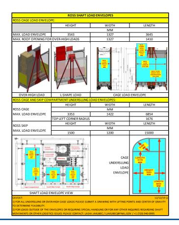
SDSD - establish the specifications of the transport cart based on largest objects (L cryostat pieces, APAs)
