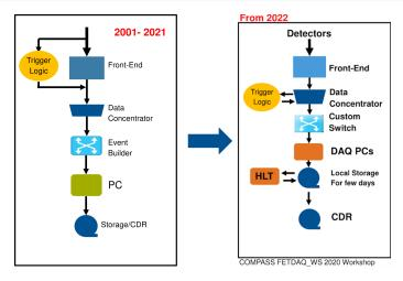
Future: Splitting the continuous data stream at the level of the Data concentrators for DAQ and trigger logic.
