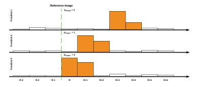
A hit in an image of an reference detector marks the image as start image. These image number is subtracted from the surrounding images.  $\rightarrow$  the maximum multiplicity shows the CTC value.
