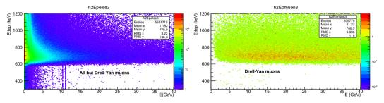
Cannot reduce the hit multiplicity with a cut on the amplitude with a FI detector
