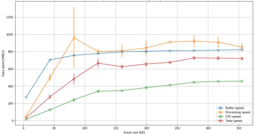
DAQ Speed Test - Basic test designed by Antonin
