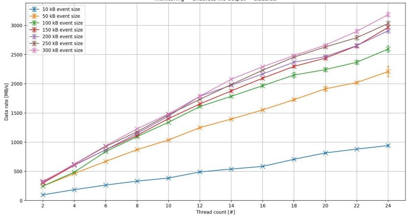
DAQ speed measurement using NUMA-aware thread management monitoring = enabled, file output = disabled
