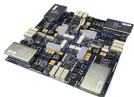
Custom made Low Voltage Power Supply (LVPS) system developed for the ATLAS – TileCal detector of the LHC
