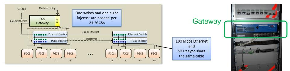
This gateway makes the interface with the control room through the general control infrastructure.
