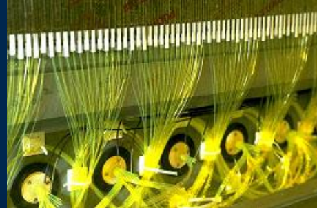
WLS optical fibers routing. Fiber aluminization done in Lisbon
