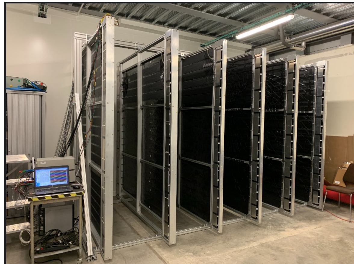
ToF panels assembled at CERN
