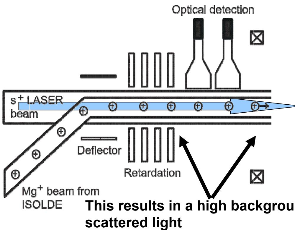
Within the light collection region the ion beam should have zero divergence (parallel beam)
