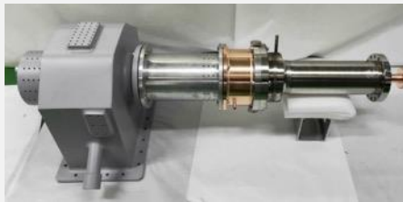
High power test of one 650 MHz fixed coupling input coupler reached 150 kW SW (corresponding to 400 kW TW at the window). Another coupler's window broke due to excess ceramic heating. New window and two variable couplers in fabrication.
