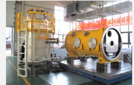
Cryomodule and valve box for two 650 MHz 2-cell cavities etc. Module assembly and beam test at PAPS in 2020.
