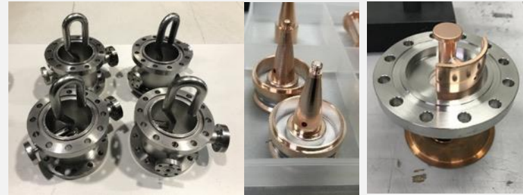
Four high power HOM couplers fabricated and low power tested with cavity. Three will mount on the 2-cell cavities. Vertical test soon with the cavity to verify the notch properties. High power test (1 kW) at RT and 2 K planned with special rigid coaxial line.
