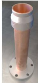
Pumping out pipe
