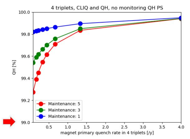
One magnet quenching implies the 5 neighboring magnet have to quench, actual number of quenched magnets is 6 times higher
