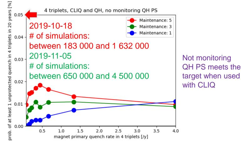
One magnet quenching implies the 5 neighboring magnet have to quench, actual number of quenched magnets is 6 times higher
