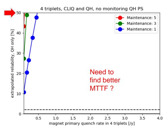
One magnet quenching implies the 5 neighboring magnet have to quench, actual number of quenched magnets is 6 times higher
