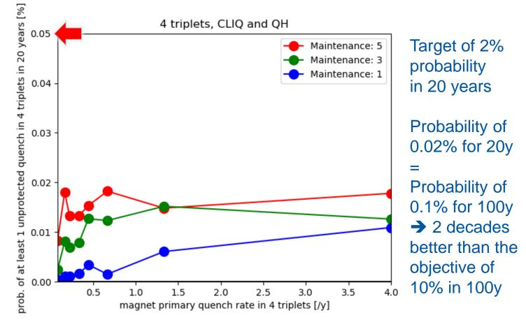
One magnet quenching implies the 5 neighboring magnet have to quench, actual number of quenched magnets is 6 times higher
