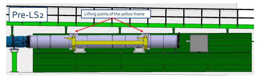
In operating conditions, the yellow lifting frame is hanging from the dump. It can't move longitudinally, because of the grey supports. If the dump moves, it will slide inside the yellow frame, so the dump's centre of gravity will not be centered between the lifting points of the yellow frame.
