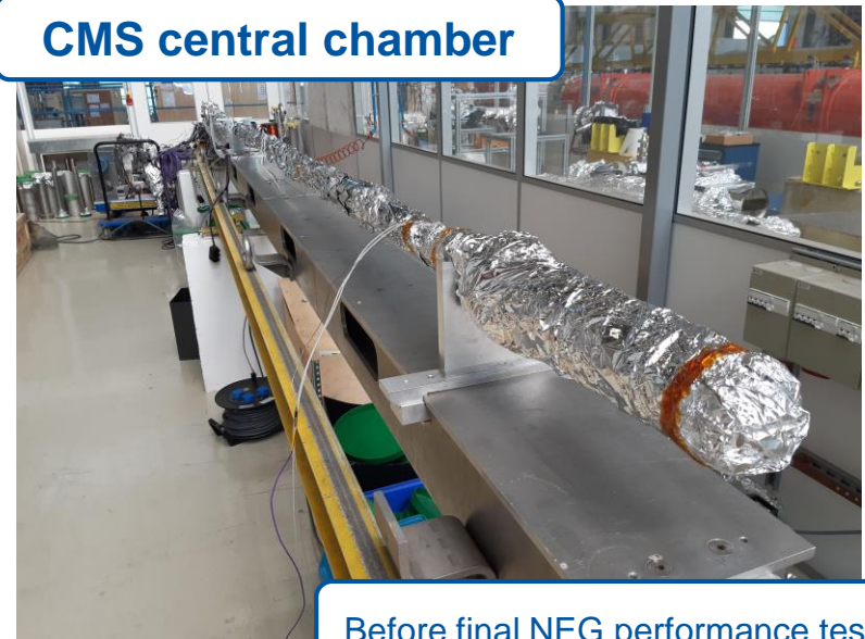
Before final NEG performance test
