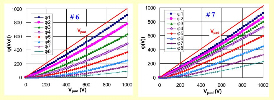
Detectors with 1 mm thickness: topology with 8 rings allows reduction of the electric field near sensitive p-n junction – main task! Distribution is controlled by VTS design
