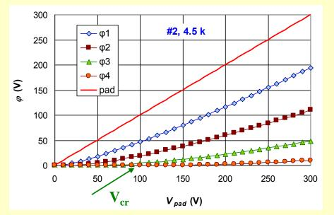
$\varphi$  starts to rise at  $V_{pad} = V_{cr}$  $V_{cr} \uparrow as \rho \downarrow$
