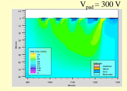
As  $V_{pad}$  increases, holes are extracted inside the gaps
