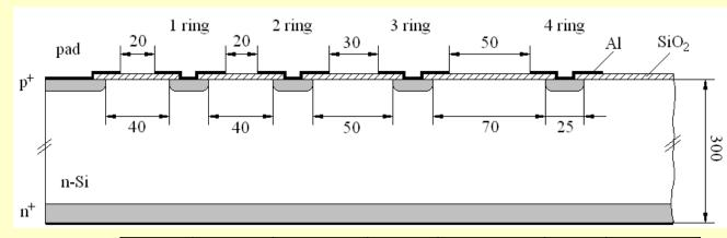
Our standard test structure: p<sup>+</sup>-n-n<sup>+</sup> 4 floating rings
