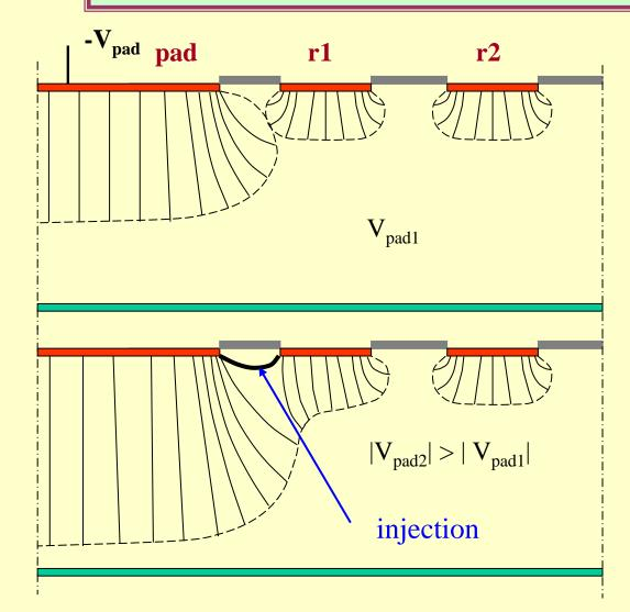
**Potential stabilization**: hole transfer to the ring + hole injection in the gap **Criteria for potential** stabilization at the ring -✓ trajectory between the rings for hole injection from the ring with lower negative potential; ✓ low leakage in the gap:  $I_{leak} < I_{gen}$  near the ring (individual for rings, less sensitive gap pad-ring maximum I<sub>gen</sub> near pad; interface properties)
