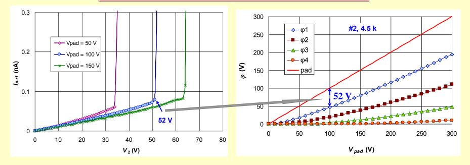
✓ Potential difference at the gap equals to the threshold voltage V<sub>th</sub> at which injection starts →
