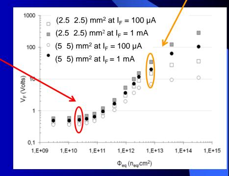
When the active area is reduced by 4 sensitivity is increased by 1.5
