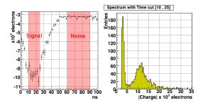
For lower voltages signal-landau shifts to lower values. The procedure works nonetheless: Example spectrum for  $150 \,\mu\text{m}$  thick sensor irradiated up to  $10^{15} \,n_{eq}$
