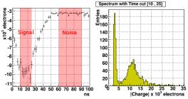
For lower voltages signal-landau shifts to lower values. The procedure works nonetheless: Example spectrum for 150 µm thick sensor irradiated up to 10<sup>15</sup> n<sub>eg</sub> @100 V:
