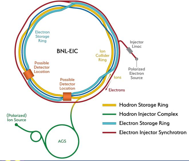
Add an electron injector complex with Rapid Cycling Synchrotron
