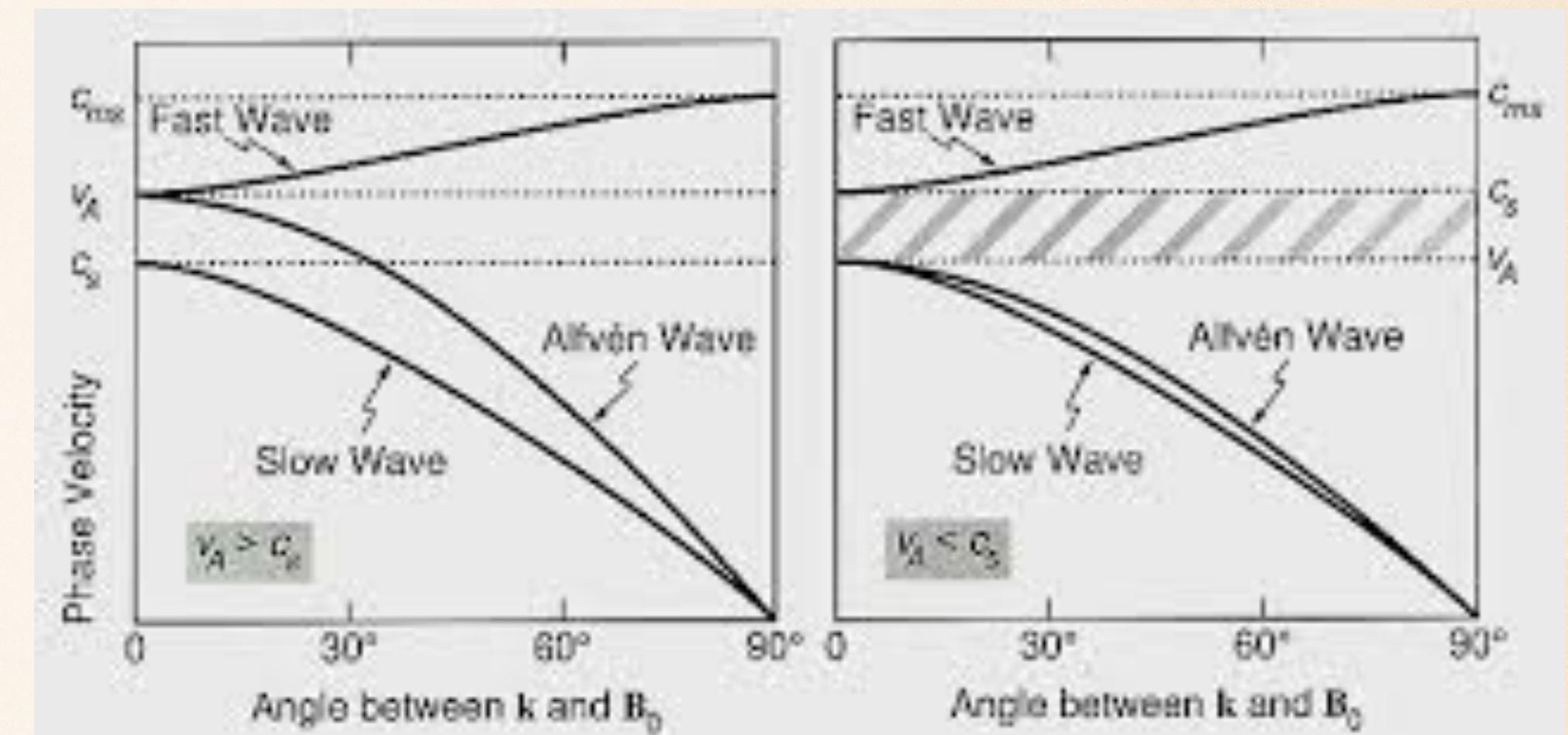
"In the absence of magnetic field the fast magnetosonic wave reduces to normal speed of sound the slow magnetosonic and the Alfvén waves become zero."
