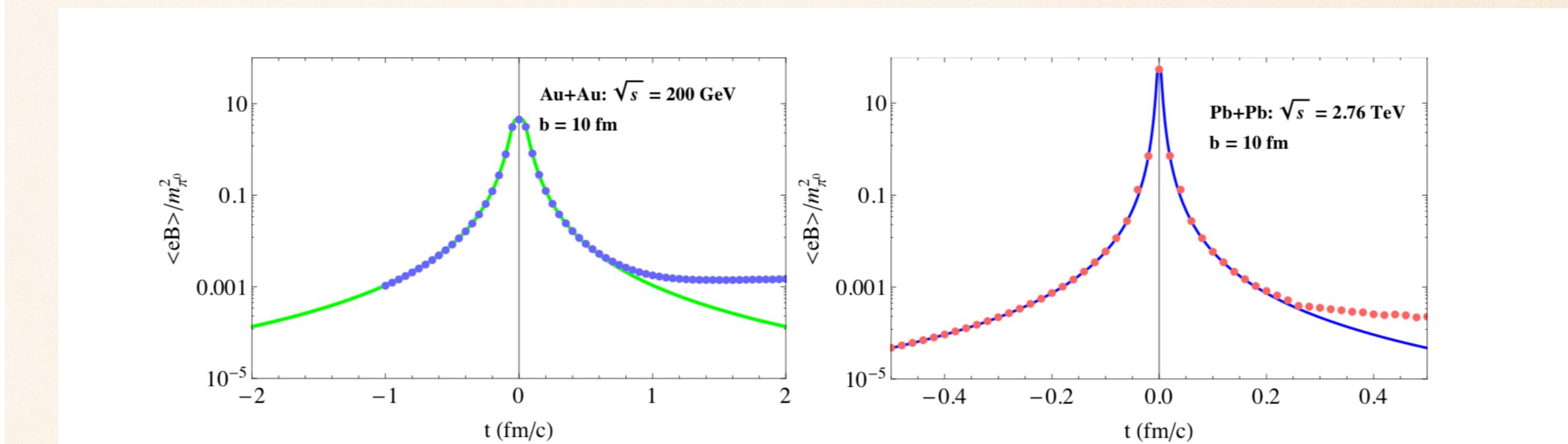
Electro-Magnetic fields are strongest during the early stage of heavy ion collisions
