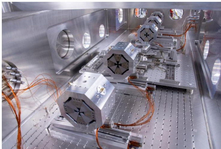
Fig. 24: Inside view of the ACHIP experimental chamber in SwissFEL. Permanent magnet quadrupoles are used to focus the electron beam, and the accelerating structure can be mounted on a hexapod.
