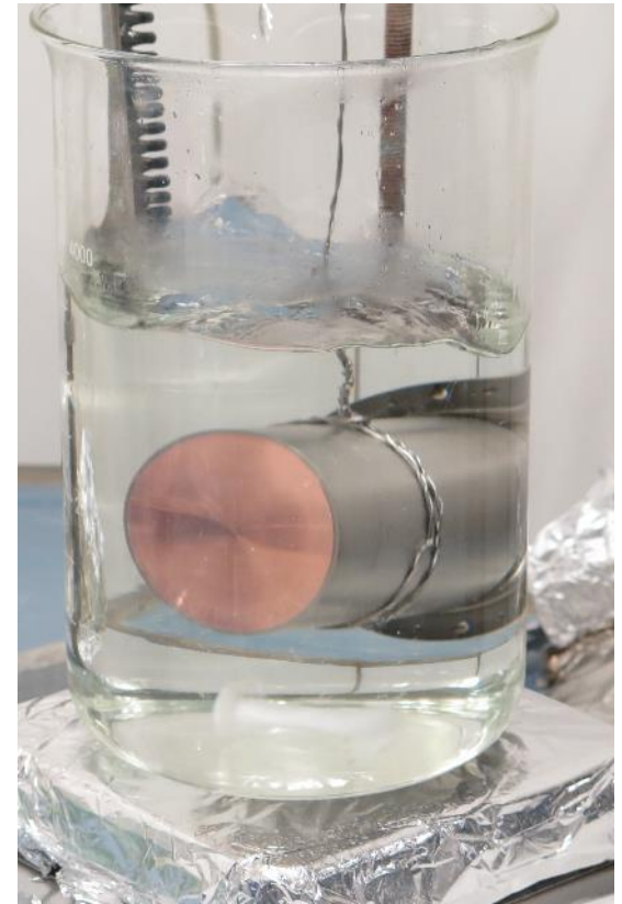
During SUBU chemical polishing
