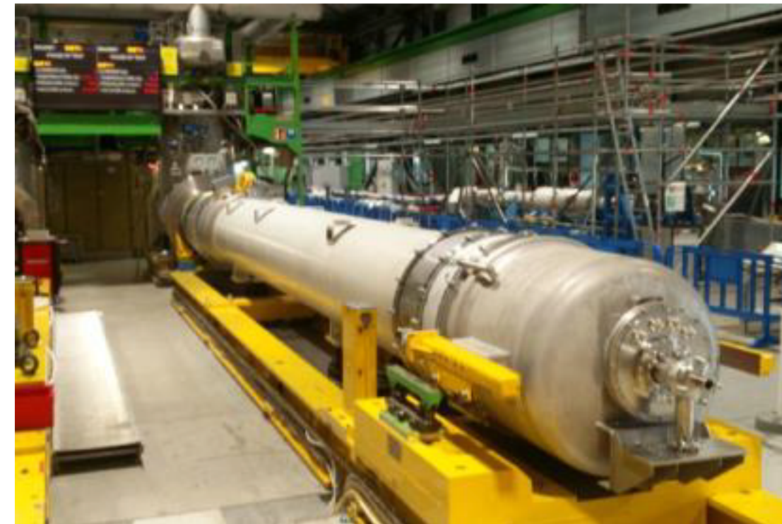
from LHC technology 8.3 T NbTi dipole
