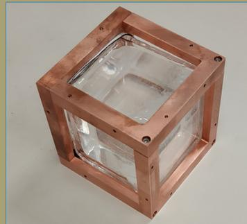
Top: NaI(Tl) crystal encapsulated in copper cage for SiPM matrices support.
