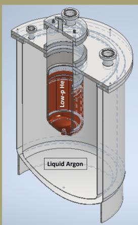
Left: simplified sketch of the ASTAROTH detector. The inner copper chamber, hosting the crystals, is immersed in a LAr bath within a closed dewar.
