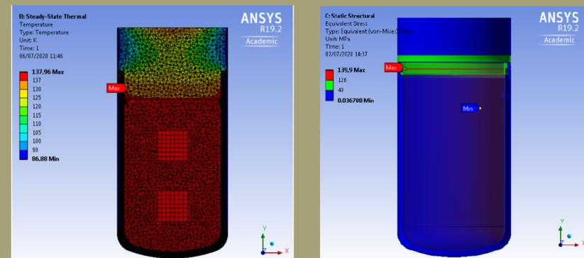
Thermal and mechanical FEAs of the ASTAROTH dual-wall copper box, highlighting the optimal temperature uniformity in the main volume (Left) and the stress map in most loaded areas (SS thermal bridge, Right)
