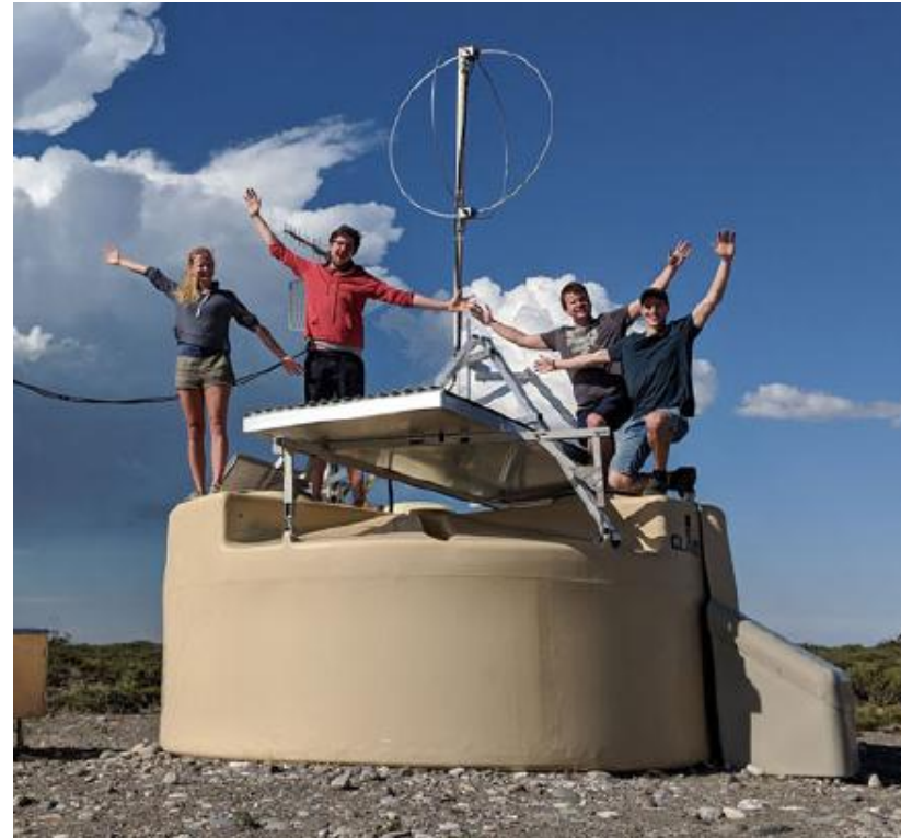
Water-Cherenkov station with new scintillator detector (SSD) and new radio antenna (RD)
