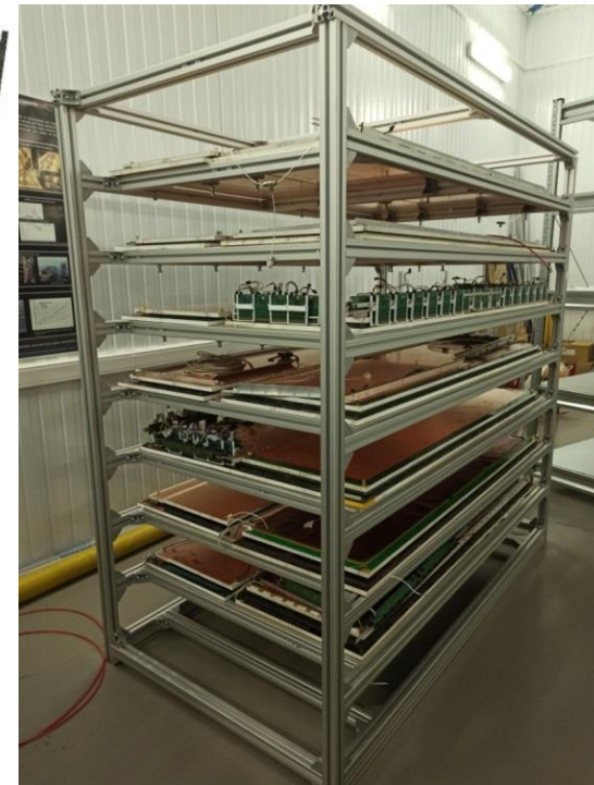
Setup of GEM detectors for cosmic tests
