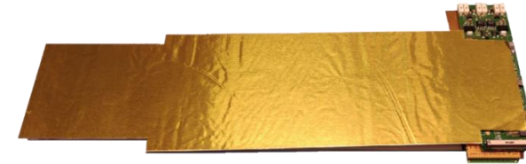
Assembled modules are covered with aluminum shielding
