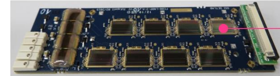
Front-end Board with 8 STS XYTER ASICs
