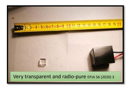
$ZnWO_4$  crystal = 10 x 10 x 10 mm<sup>3</sup> (detector of reduced dimensions to investigate neutron single-scattering)
