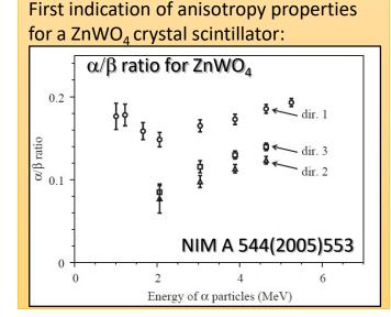
**ZnWO**<sub>4</sub> anisotropic scintillator: a very promising detector (NIMA544(2005)553, Eur. Phys. J. C 73 (2013) 2276): i) very good anisotropic features; ii) high level of radiopurity; iii) high light output, that is low energy threshold feasible; iv) high stability in the running conditions; v) sensitivity to small and large mass DM candidate particles; vi) detectors with ~ kg masses feasible 5
