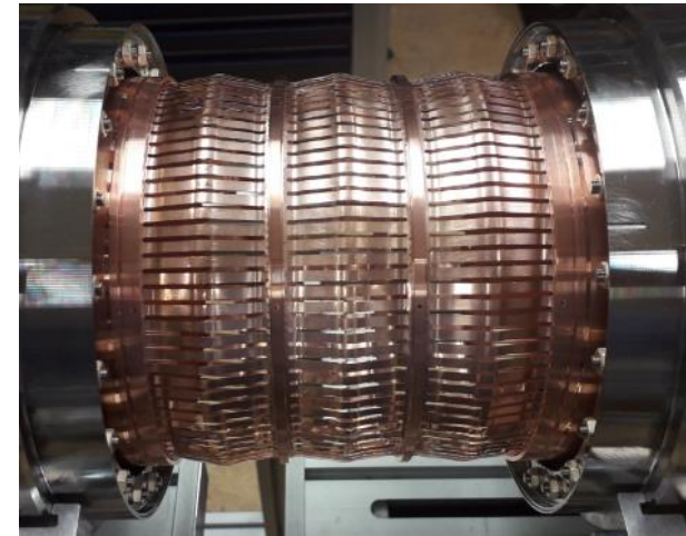
Deformable RF bridges
