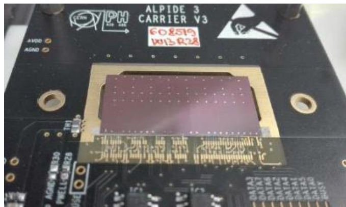
ALPIDE sensor (from ALICE collaboration) 30 \times 15 \text{ mm}^2
