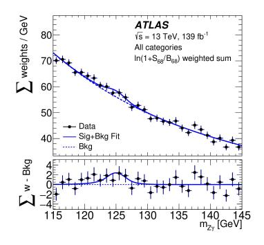
Signal + background fit (line), background only fit (dashed) and data (dots)
