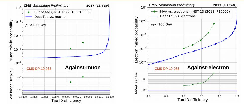
• The DeepTau against-muon (electron) classifier allows to obtain a noticeably higher rejection of  $I \rightarrow \tau_h$  fakes compared to the cut-based (MVA-based) algorithms previously used
