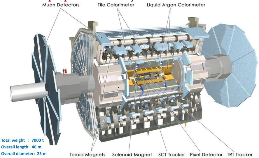
Magnetic field: 2T solenoid + (varying) toroid field
