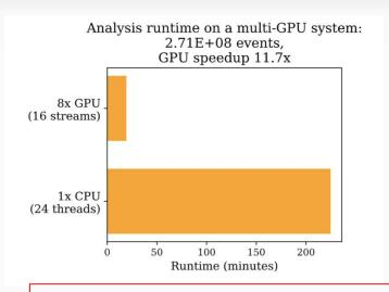
Use 8 Nvidia GTX 1080 GPUs, 2 compute streams per device → reduce the analysis runtime by a factor of 12x compared to using multiple threaded CPU
