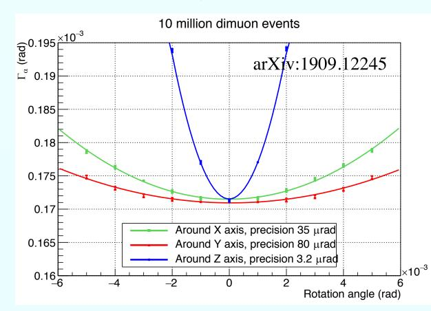
The precision on the Euler rotation angle around the y axis improves from 80 to 18  $\mu$ rad (in one hour at the Z pole) by also minimizing the correlation between  $\alpha$  and  $x_{\gamma}$ : such a rotation with respect to the natural frame mixes indeed the x ( $\alpha$ ) and z ( $x_{\gamma}$ ) information in a visible way:
