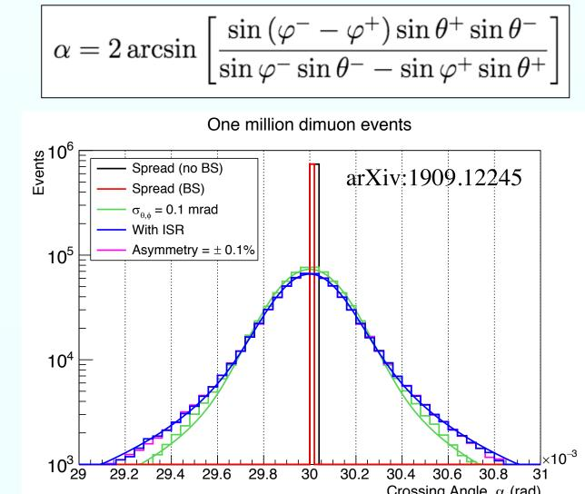
The spread of the  $\alpha$  distribution from dimuon events is smallest when the z axis (used to determine  $\theta^\pm$ ) and the x axis (used to determine  $\varphi^\pm$ ) are perfectly known. The alignment of the detector with respect to these axes can therefore be achieved with a minimization of this spread. Precisions of 3.2 (35)  $\mu$ rad on the Euler rotation angles around the x (z) axes need only one hour at the Z pole.
