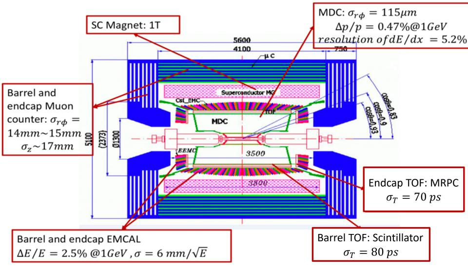
• General purpose detector at BEPCII,  $E_{cm} \approx 2-4.6 \text{ GeV}$ ,  $L_{peak} \approx 10^{33}/\text{cm}^2/\text{s}$
