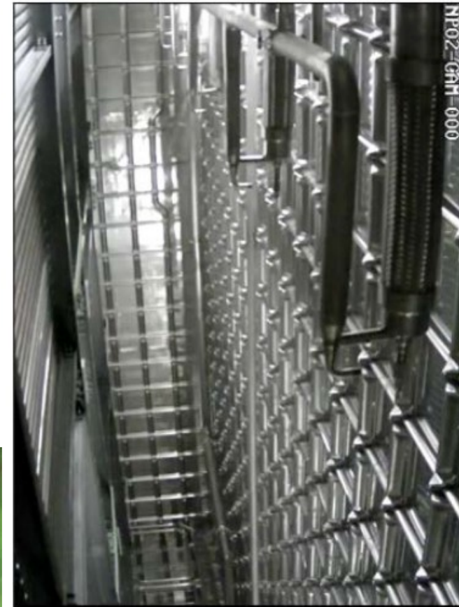
DP field cage and cryostat wall during filling
