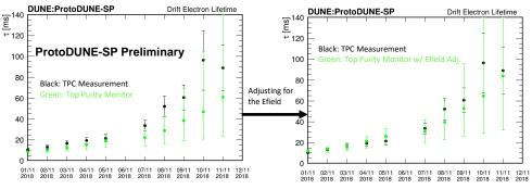
Attachment rates for impurities differ based on the electric field of the drift volume. The purity monitors operate at around 25 V/cm, while the TPC operates at 500 V/cm.
