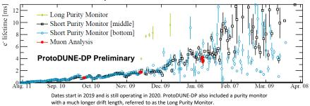
Cosmic muon measurements of the drift electron lifetime agree with the purity monitors in ProtoDUNE-DP.
