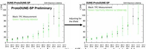
Attachment rates for impurities differ based on the electric field of the drift volume. The purity monitors operate at around 25 V/cm, while the TPC operates at 500 V/cm.
