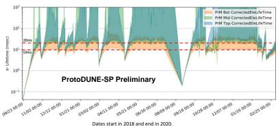
The TPC drift electron lifetime was measured directly using cosmic muons to validate purity monitor measurements.
