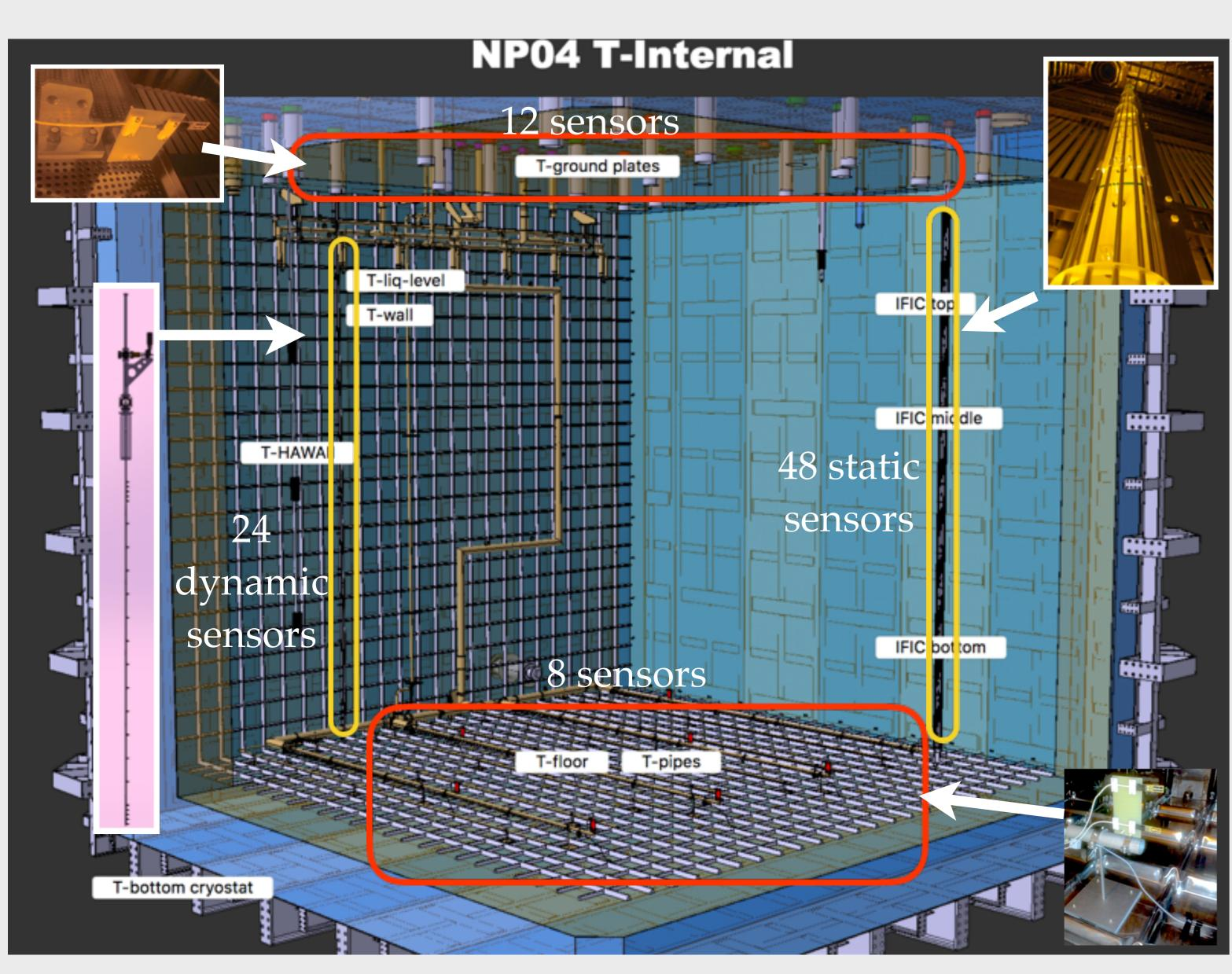
Schematic showing various temperature sensors and their location in the ProtoDUNE cryostat. The dynamic temperature profiler is shown on the left.
