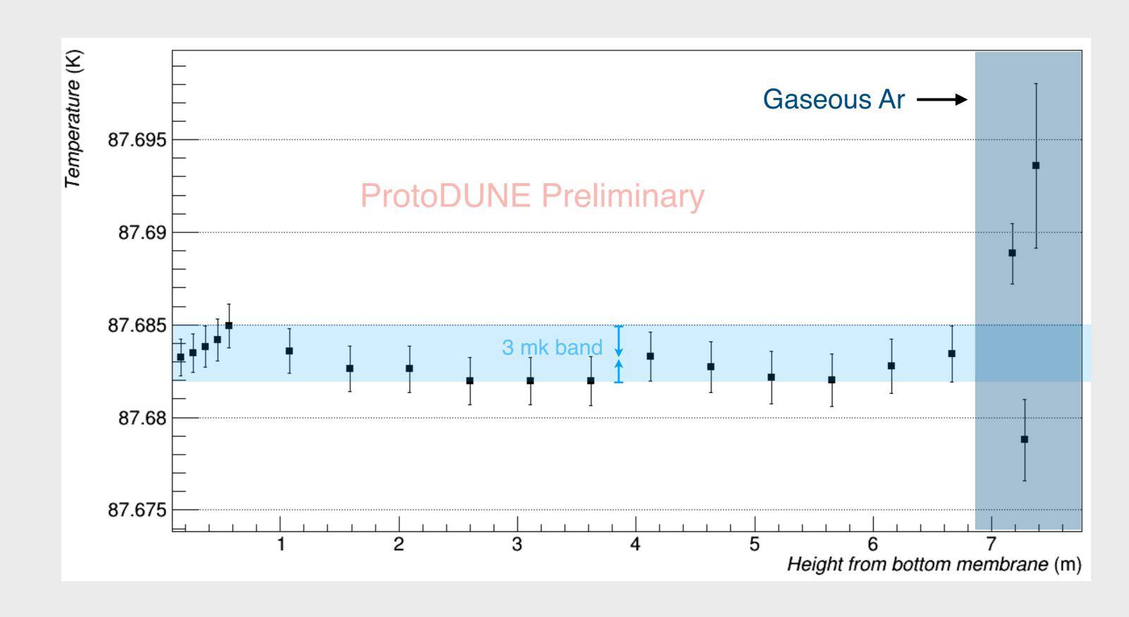
•Including the offsets corrects for residual parasitic resistance and electromagnetic noise and yields a relative accuracy of 2-3mK.
