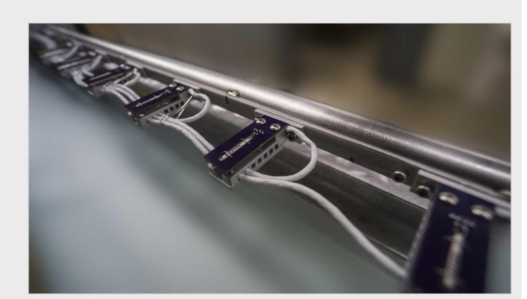
• The ability to move the dynamic profiler, allows for cross-calibration of the sensors.
