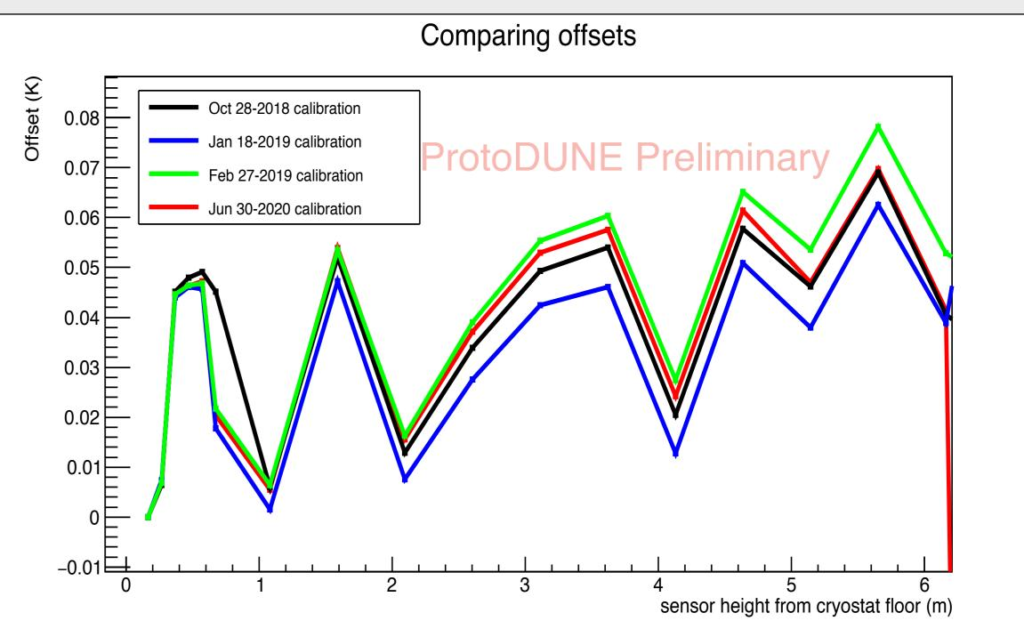
•The ability to move the sensors vertically is utilized to cross-calibrate the static sensors. The sensor values are then used to validate Computational Fluid Dynamic (CFD) models of liquid Argon in the detector.
