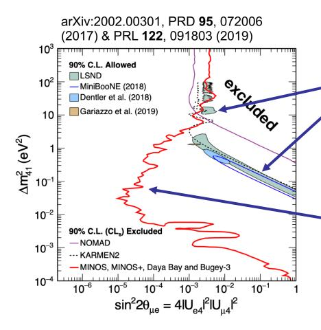
$v_{\mu} \rightarrow v_{e}$  appearance seen by LSND and MiniBooNE consistent with a sterile neutrino
