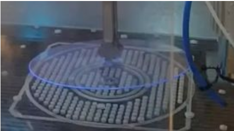
9 Legend plates machined from 180 grams PEN plate.
