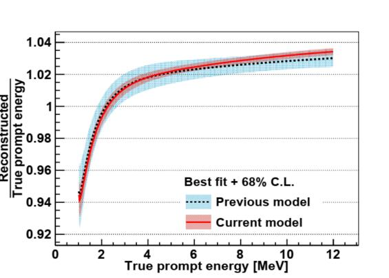
Uncertainties in the absolute energy calibration is reduced to less than 0.5% from previous 1.0% for visible energies larger than 2MeV.
