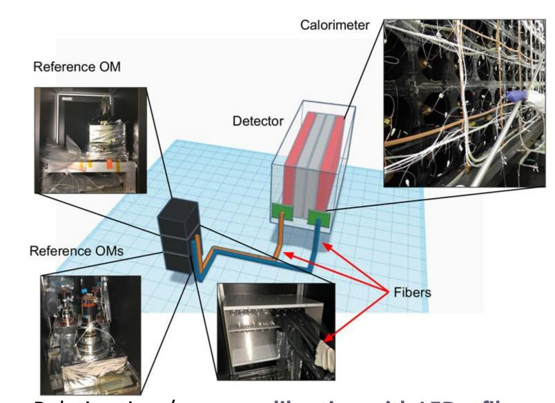
Relative time/energy calibration with LED + fibers + Absolute energy calibration with <sup>207</sup>Bi sources
