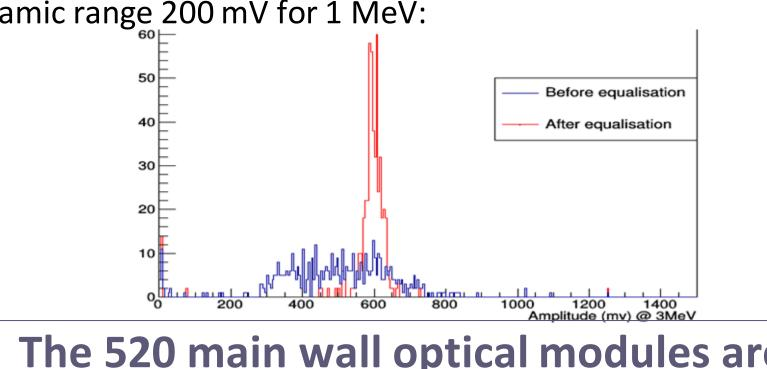
The 520 main wall optical modules are equalised with gain spread < 10%
